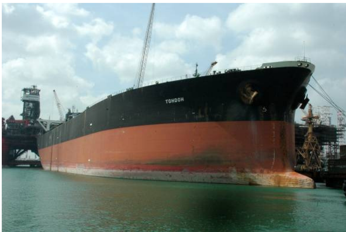
Ohdoh (ex Tohdoh), size 330mL x 59mB x 30mD on arrival at Jurong Shipyard for conversion to FPSO Kwame Nkrumah MV21
